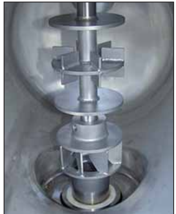
Pump-mix-turbine from mixer-settler type MST 300
