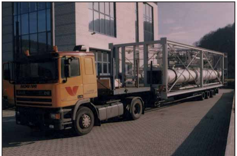
Transport of a pre-assembled skid-unit
