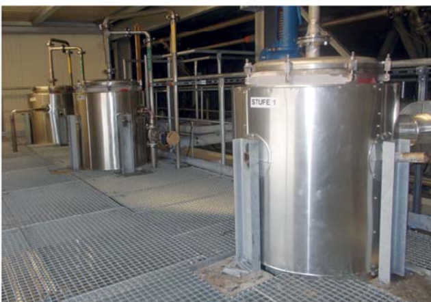
3 stage Falling-film evaporator viscous products 800kW
