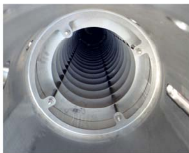
Stator mounted in column shell
