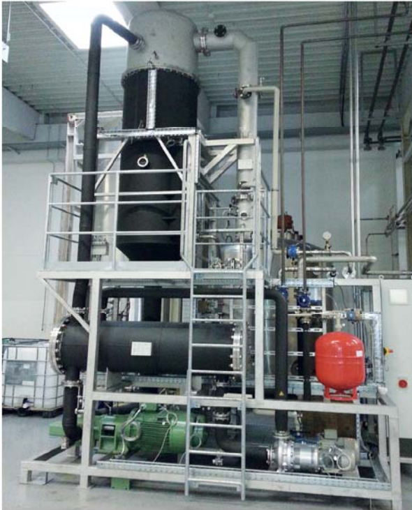
Forced circulation evaporators; separation of water from hydraulic oil. Viscosity up to 20.000 mPa s.
