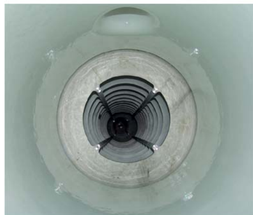
Glass lined steel column with Hastelloy C4 + C22 / PVDF Internals for corrosive solutions hydrochloric acid
