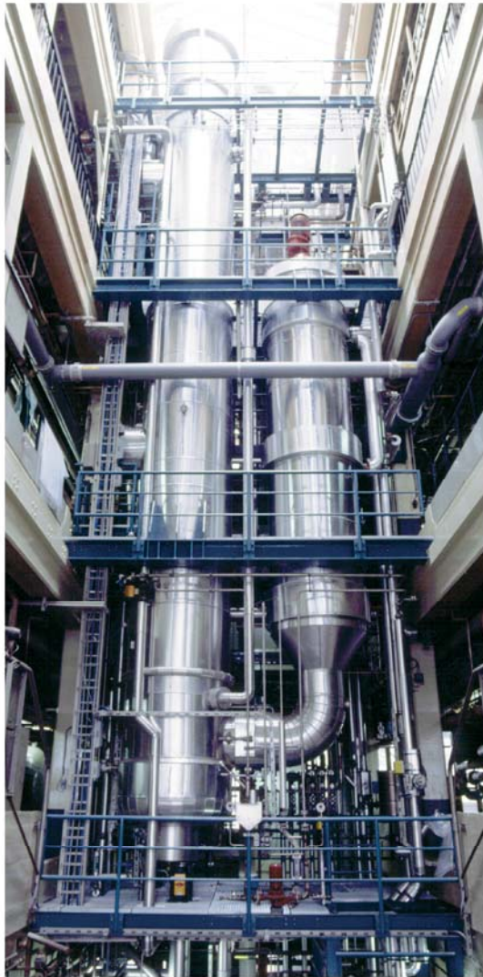
Rectification plant with thin-film evaporator (vacuum 100 Pa)
