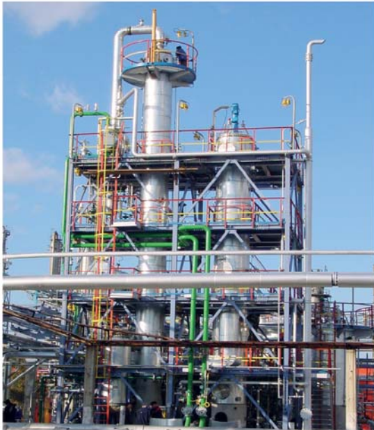
Agitated column with solvent recovery
