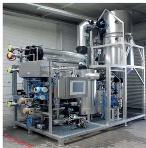
Heat-pump evaporator White Spirit, ATEX, silicone-free
