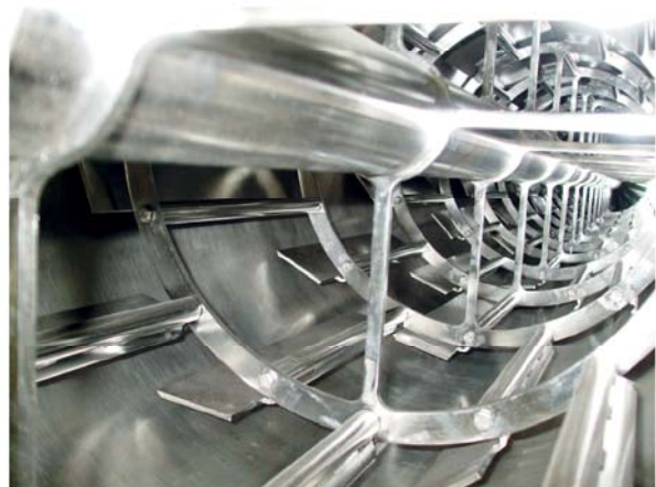
Thin-film evaporator high viscose products 6,3m 2
