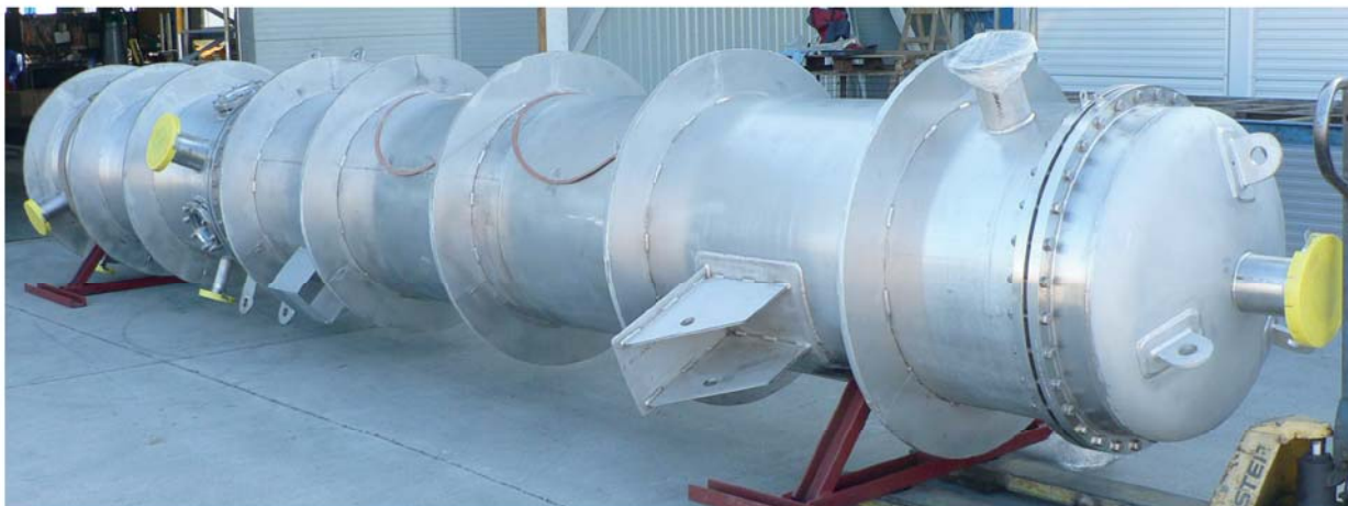
Fall-film evaporator methanol biodiesel 1150kW
