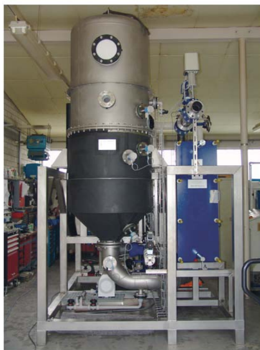
Forced circulation evaporator 84% \text{H}_3\text{PO}_4
