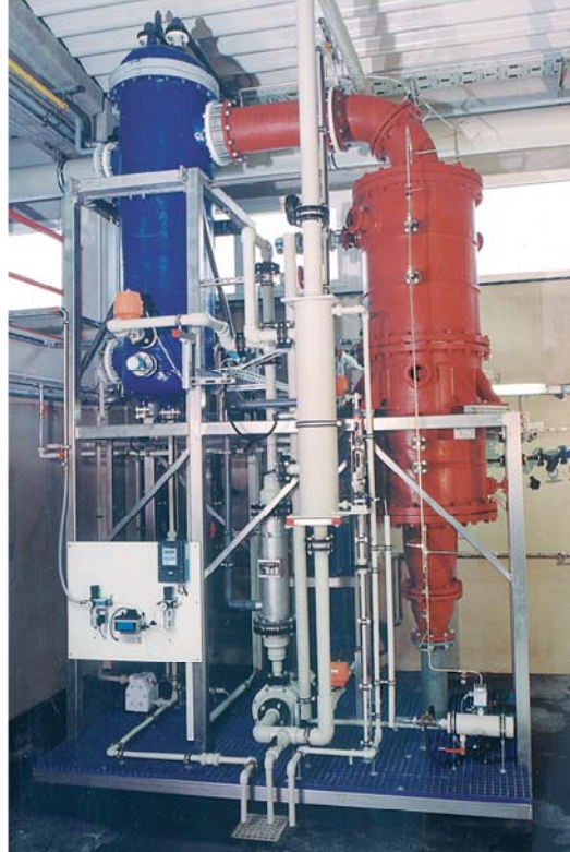
Forced circulation evaporator \text{H}_2\text{SO}_4 85% + HF
